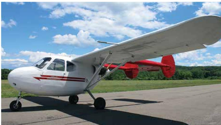
**READY FOR TAKEOFF:** Claverack member Russ Darrow's Trella T-21 experimental airplane returns to the great blue yonder for testing purposes in June after undergoing two and one-half years of restoration work by the owner. The pusher plane, with a single propeller located behind the engine, took its maiden flight in 1949 near Detroit, where it was originally constructed.
